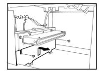
4 Remove the CCD Assy. (two shoulder screws, Three connectors)
